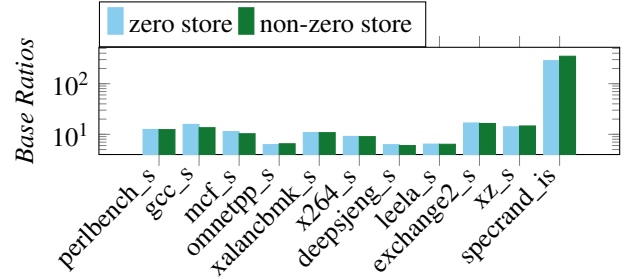
Figure 8: Performance penalty of turning off zero-store elimination on the SPEC CPU 2017 Intspeed benchmark. Disabling zero-store elimination leads to a median performance penalty of 0.8 % and average performance penalty of 0.27 %.
